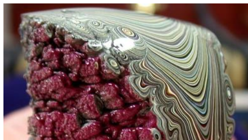
November's What in the World? photo showed a specimen of Fordite , also known as Detroit agate or Motor City agate . It is old automotive paint which has hardened sufficiently to be cut and polished. It was formed from the buildup of layers of enamel paint slag on tracks and skids on which cars were hand spray-painted (a now automated process), which have been baked numerous times. In recent times the material has been recycled into jewelry.
